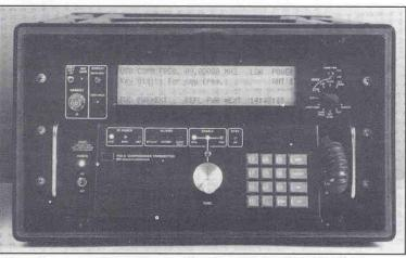
Figure 2. An ionosonde transmitter. Photo courtesy Gerald Oicles/BR Communications, Sunnyvale, CA
